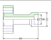
Process side oval flange with SW end connection for manifold
